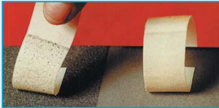
Blasting with Blast-One SpeedBlast™ on right and Blasting with Coal Slag on left. Note the embedment levels found on this simple test.
